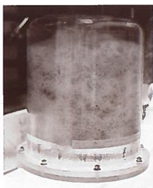
A 46-DAY-OLD CULTURE OF HAIRY ROOTS OF TAGEAS PATULA , A SPECIES OF MARIGOLD. THE REACTOR IS 20 LITERS AND THE ROOT WEIGHS APPROXIMATELY 4 KG.
